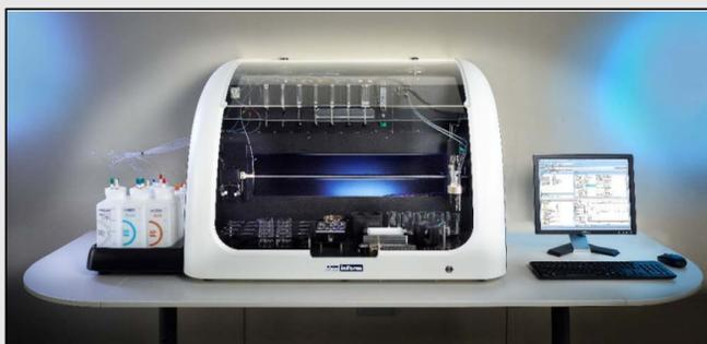
Figure 1: **Sirius inForm** platform used for biphasic dissolution testing
