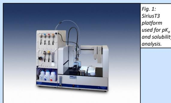
Fig. 1: SiriusT3 platform used for pK<sub>a</sub> and solubility analysis.
