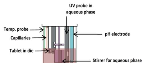
Figure 1: Probe set on the Sirius inForm platform showing UV fibre-optic probes for quantitating drug in aqueous media
