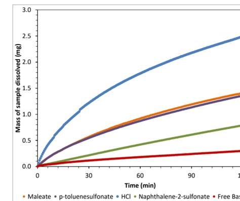
Figure 5: Dissolution profiles of free base, HCl, p-toluenesulfonate, maleate and naphthalene-2-sulfonate salts
