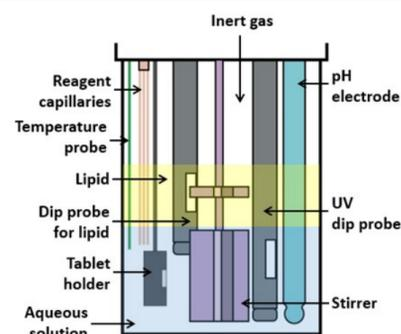
In Sirius inForm, temperature and pH are controlled in situ and media are added automatically. Stirrer paddles agitate both the aqueous and organic layers by immersing one in each layer.
